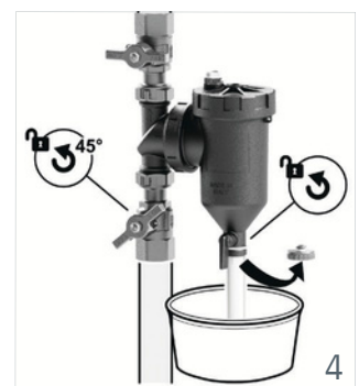
4. Slightly open the shut-off valve upstream and allow water to flush the inner parts
